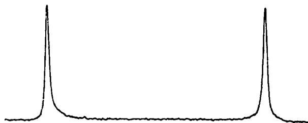
FIGURE 2 D-NMR spectrum of \text{C}_6\text{D}_6 in 17% PBLG/m-cresol at 302 K. The line splitting is \Delta\nu_{eq} = 724 \text{ Hz} .
